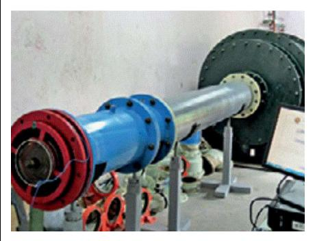
CHENNAI: A team of 25 faculty members and students from the <u>ocean</u> engineering department in Indian Institute of Technology Madras have begun testing a prototype of a turbine they have developed which converts wave energy into electricity. The 'impulse' turbine works with a unidirectional rotor powered by a generator. The system will be tested in oceans by the end of the year.
